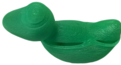
Fig. 5.6 The toy duck used as a case study, which exhibits a fabrication defect.
