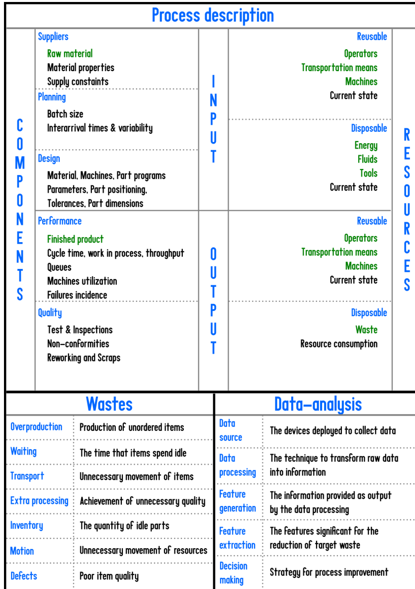
Fig. 3.1 The schematic of the methodology used to develop this work. Black color represents information; green color is used for physical quantities.
